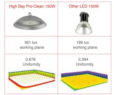
Room width 100m Room length 100m Room height 10m Fixture Qty 225pcs Fixture spacing 6.7m
