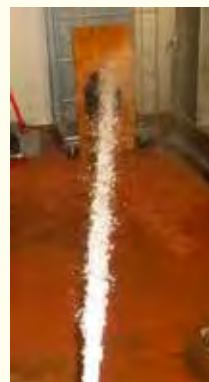
Picture 24: IP test - WATER
