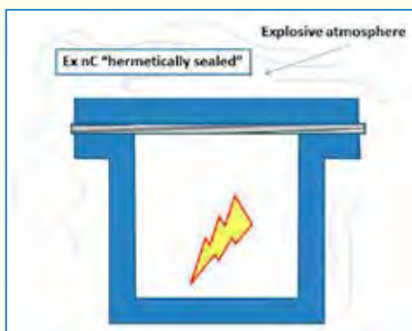
Picture 13: type of protection Ex nC (hermetically sealed)
