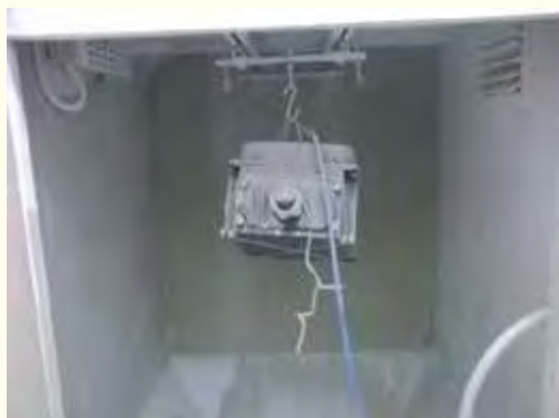
Picture 23: IP test - DUST
